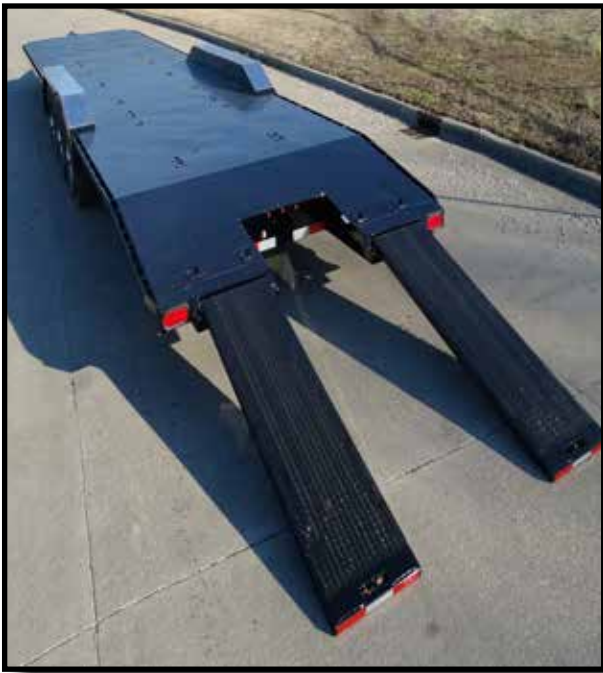
35' Double Car Hauler with options: drive over fenders and full outriggers, treadplate on full fender, and extra D-Rings.
