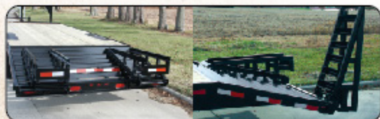
Self-cleaning, 240 lb. spring loaded ramps lift with your fingertips!
